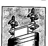
**Alternate Pilaster Mounting**
